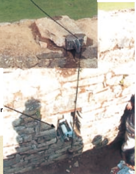
Long-span extensometer crossing the Plaza from below the Intihuatana to Residence block.
