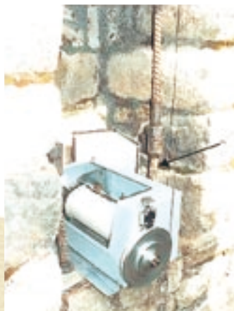
Long-span extensometer crossing the Plaza from below the Intihuatana to Residence block.
