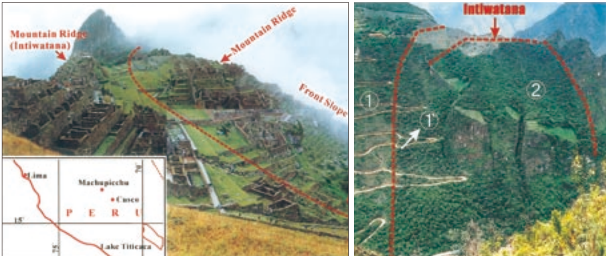
Photo of Machu Picchu and estimated landslide block boundaries passing through the monument.
