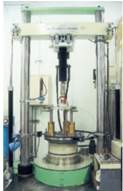
Ring shear apparatus with transparent sample box
