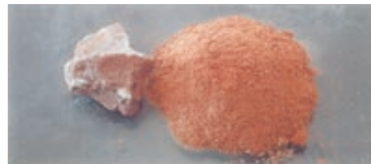
Conglomerate (left) and siltstone (right) after a few minutes of immersion in water. Siltstone is vulnerable to water intrusion.
