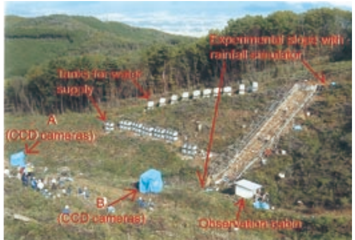
Artificial rainfall experiment site for triggering landslide on natural slope
