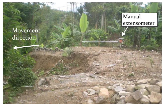
Figure 2 A manual extensometer could detect a collapsed slope and warns the community to evacuate.
