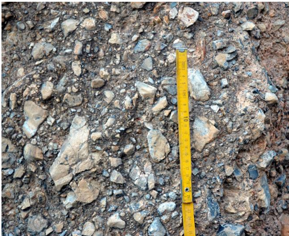
Figure 92. Typical grain-size composition of crushed granite (above) and metasediments (below) of the Kokomeren rockslide right-bank body lower part
