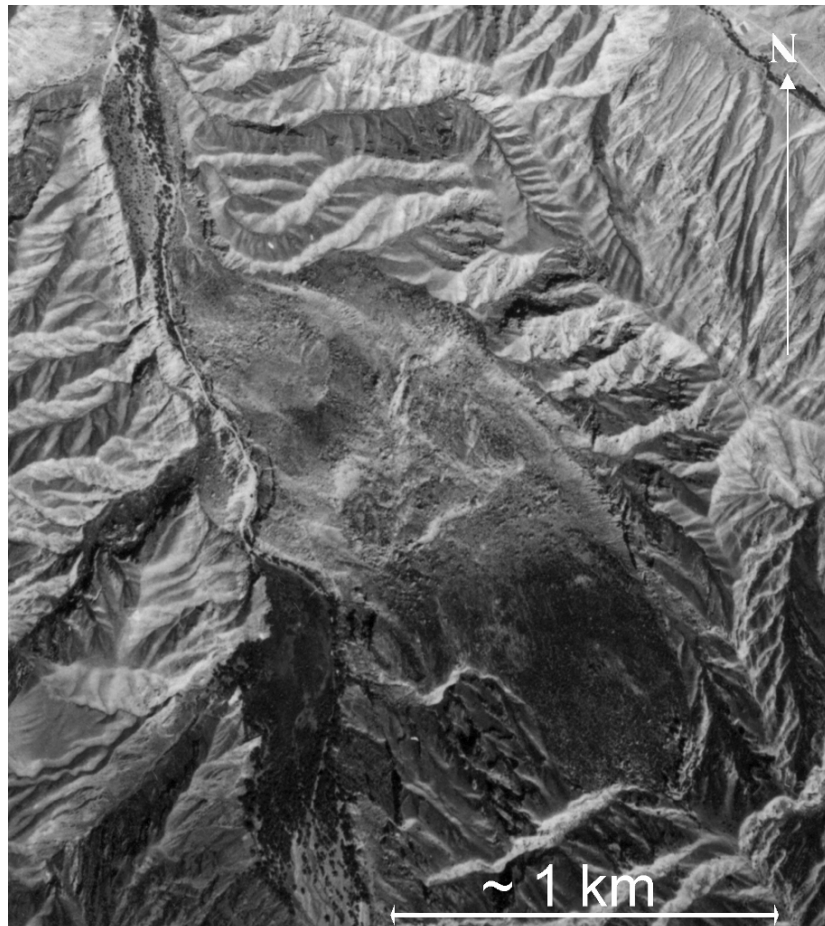
Figure 185. Aerial photo of Lower Ak-Kiol rockslide
