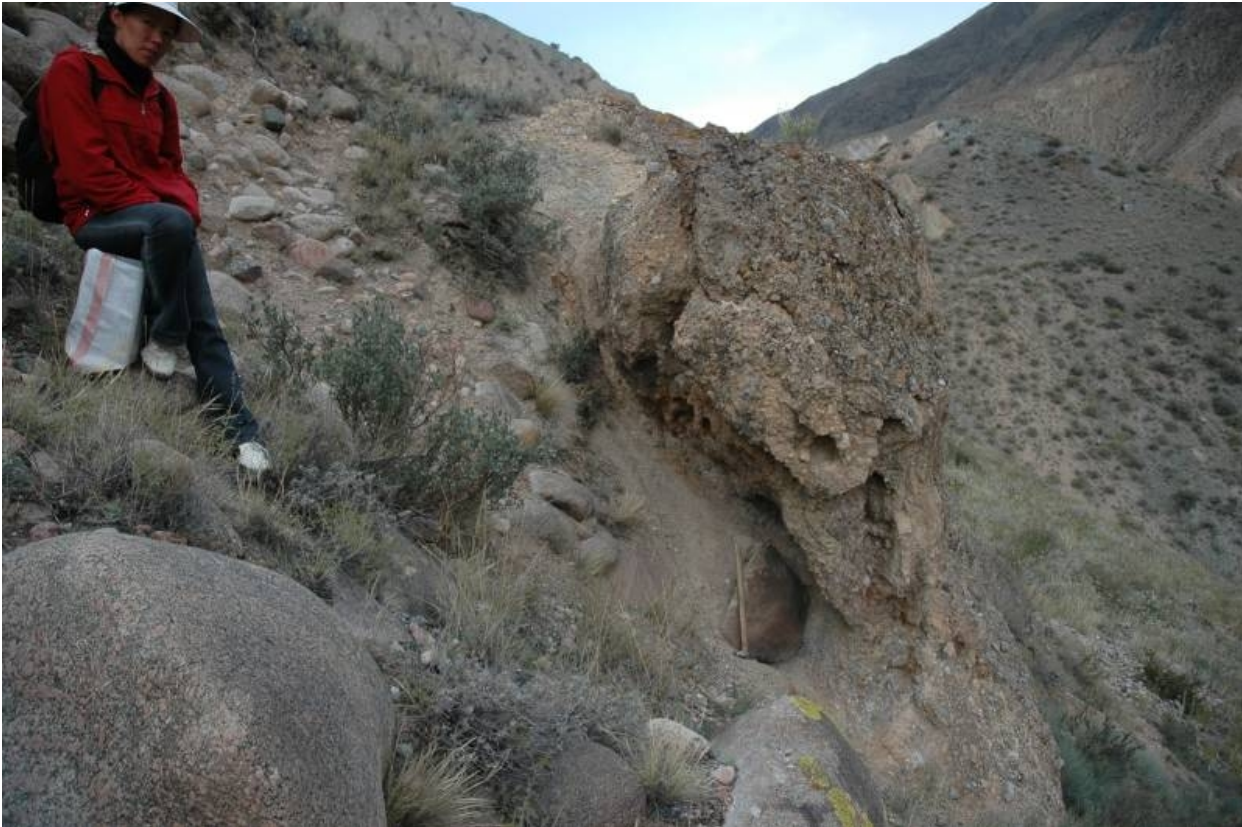
Figure 137. Contact of the cemented rockslide breccia and bouldery alluvium of the Kokomeren River valley right bank
