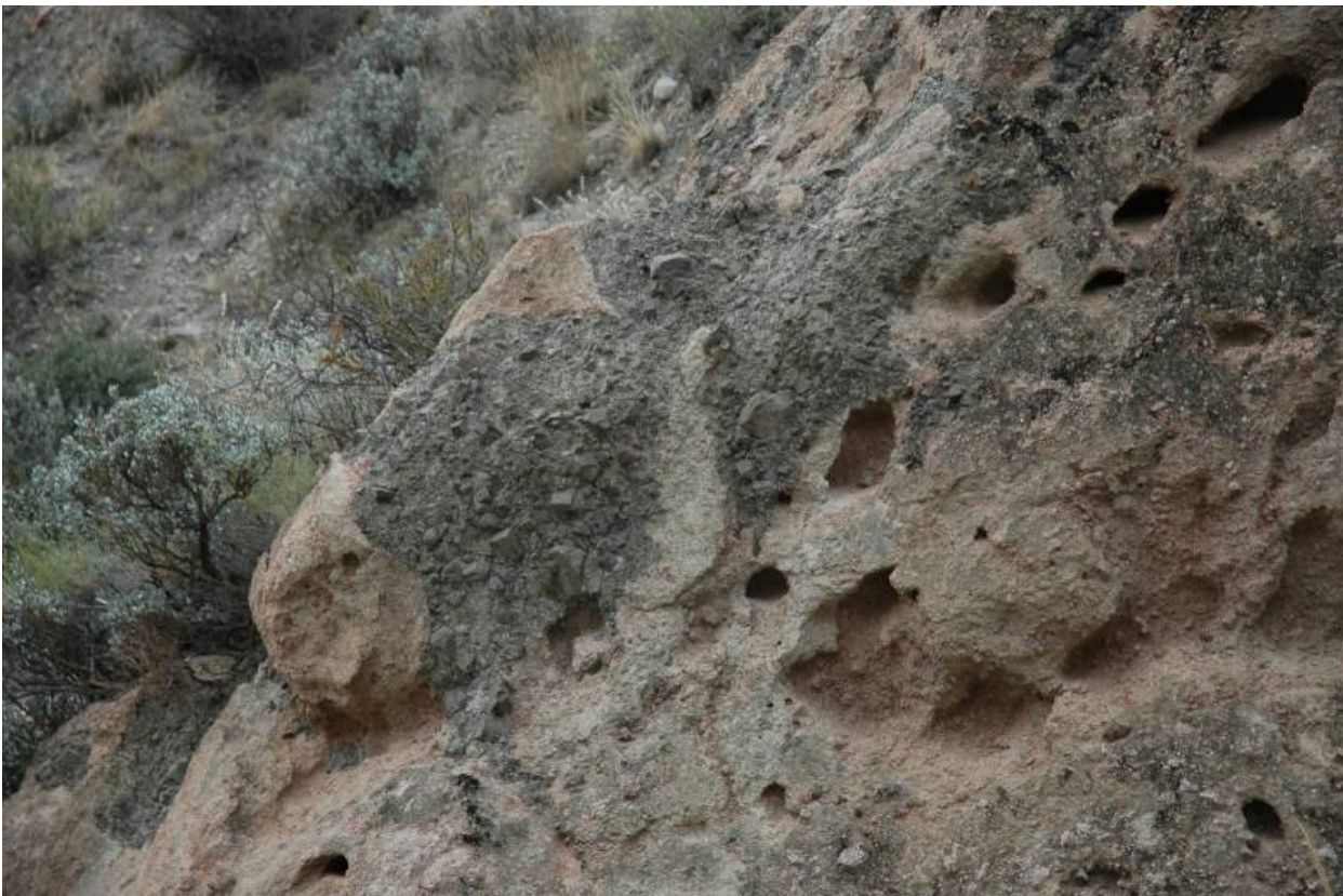
Figure 138. Meter-size succession of crushed but unmixed granites and metasediments They form cemented breccia at the frontal edge of the right-bank part of the Kokomeren rockslide
