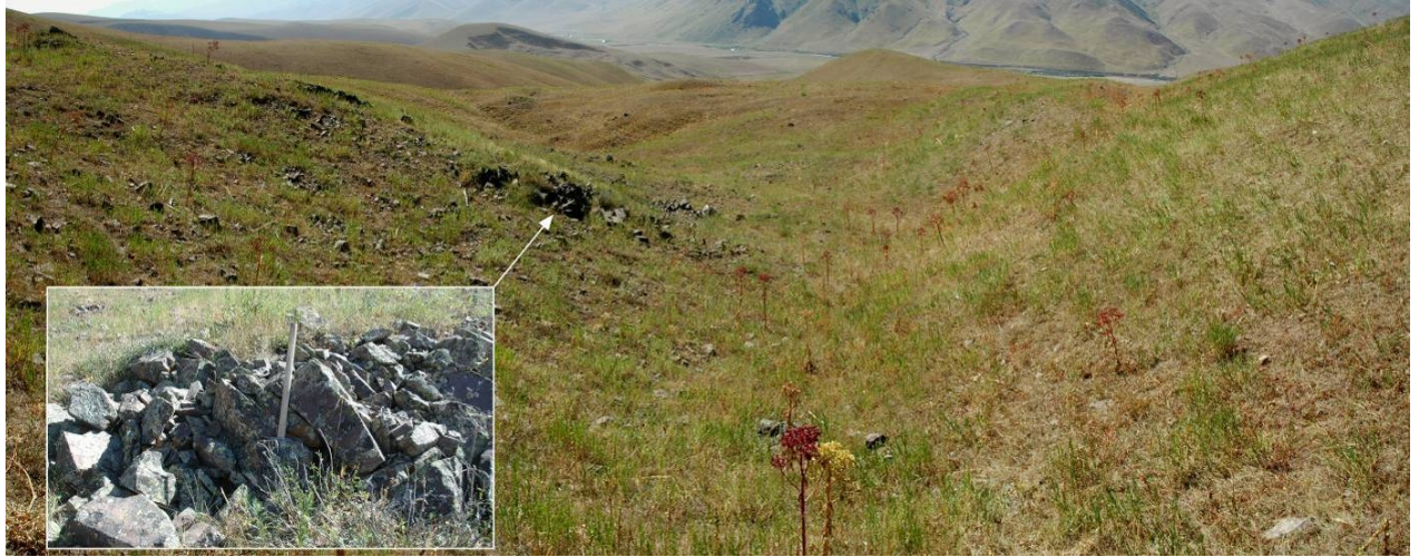
Figure 117. Sharp boundary between the inner zone of the rockslide body composed of crushed bedrock (left, see also the inset) and the outer zone composed of weathered superficial material (right)
