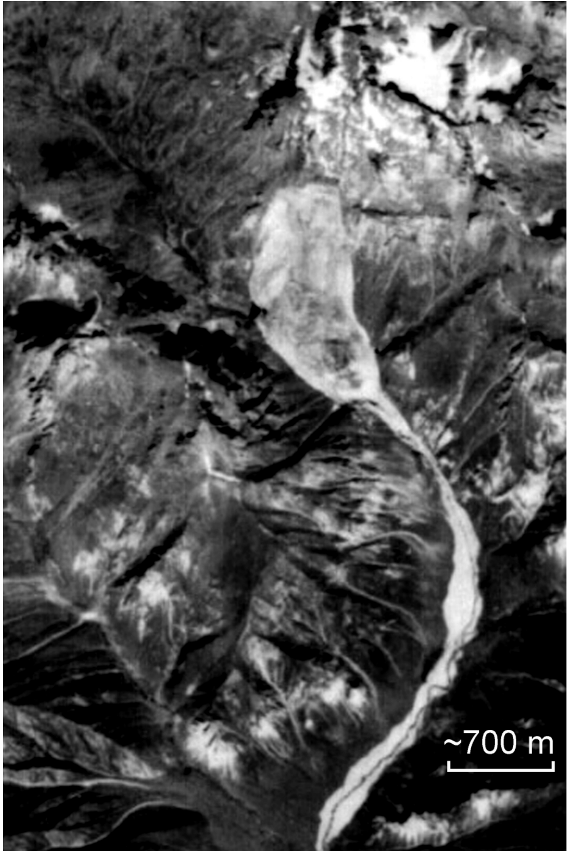
Figure 29. Rockslide in the upper reaches of the Belaldy creek caused by the 1992 Suusamyр earthquake River valley downstream was affected by the debris flow that occurred about one year later. Zoomed fragment of the KFA-1000 space image
