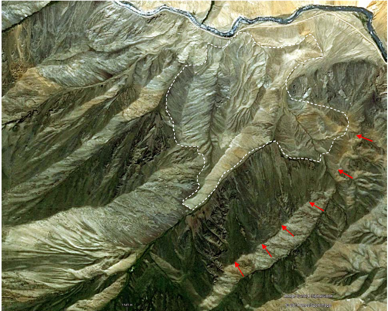
Figure 155. High resolution space image of the "Displaced Peneplain" rockslide. White dashed line marks deposit boundary; red arrows – the headscarp
