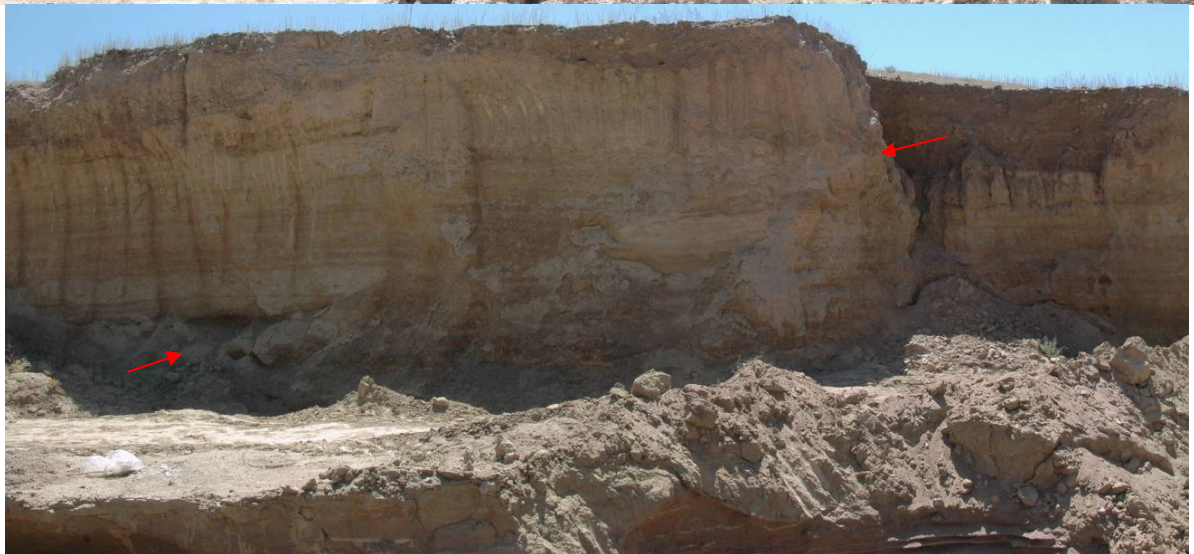
Figure 20. Above – upper (southern) rupture plane; below – lower (northern) rupture plane Dashed arrows mark possibly bifurcated rupture surfaces
