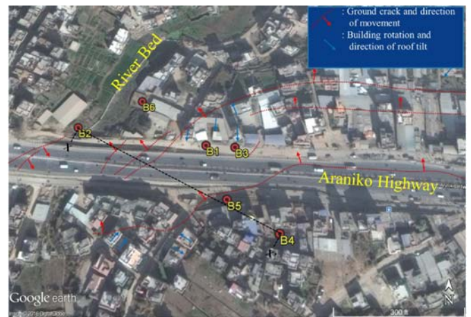
Figure 5 Location of sub-soil exploration points and landslide cross section used in the numerical analysis.
