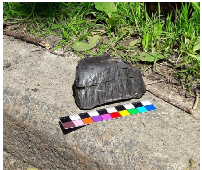
Figure 3. Slickenside in Oxfordian clay (borehole 7-K)
