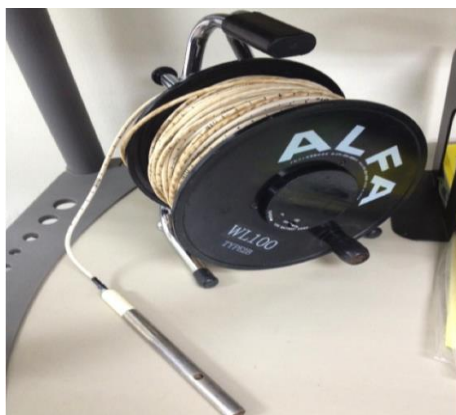
Fig. 13 Underground water level meter (Photo by author, 2013)
