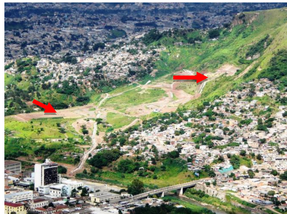
Fig. 11 In Berrinche, soil was removed from the top and compacted at the soccer field area, acting as a counterweight. (Taken by Froilán Castro, 2013)
