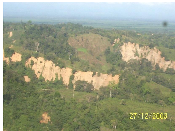
Fig. 4 Landslides on fault planes because of the December 25, 2003 earthquake, M_w=6.2 in Puerto Armuelles (taken by Eduardo Camacho in 2003)
