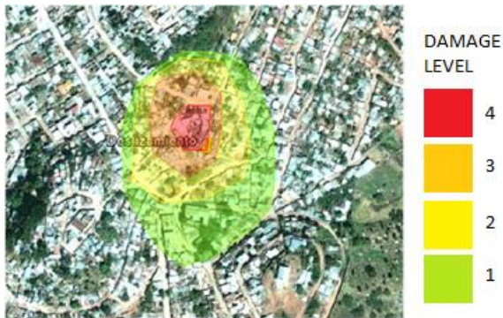
Fig.2 Illustration of the impact of a previous landslide that occurred in the area. The higher the number of damage level according to the legend, the higher the severity of the impact in a specific zone
