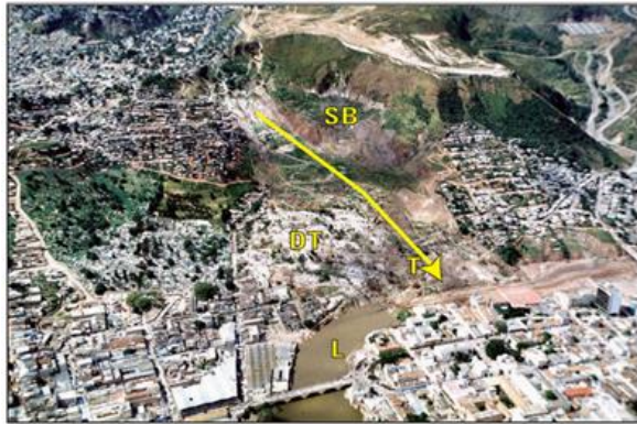
Fig. 1 Aerial view of the land called the Berrinche, followed by subsidence / rotational flow. The arrow indicates the direction of displacement of the whole landslide body. "T" denotes the sliding to the river; the "L" indicates the lake dammed by landslide. (Harp et al., 2002)
