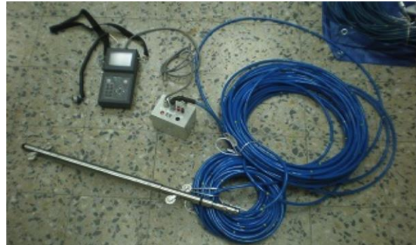
Fig. 14 Inclinometer. (Photo by author, 2013).
