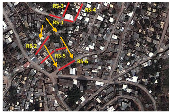
Fig.6 Illustration of the seismic refraction profiles that were made to study the layering of the zone (Source for basemap: www.google.com/maps)
