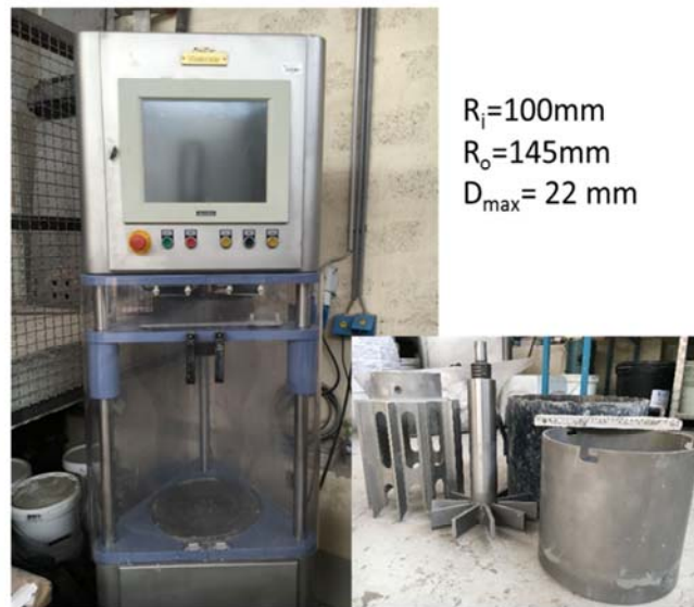
ConTec Viscometer 5, Shear rate controlled coaxial cylinder rheometer,
