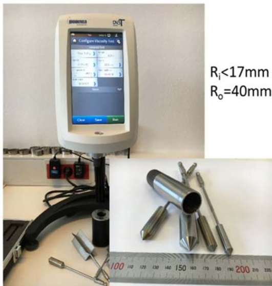
DV3THB, Brookfield – shear rate controlled coaxial cylinder rheometer
