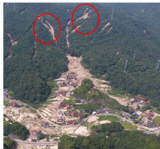
In June, 2018, a seasonal "Baiu" front extending over the western Japan became stationary causing thousands of RRLLs including this one in Yasuura, Hiroshima. The debris mass from 150m altitude slid over a 1 km distance killing one lady.
