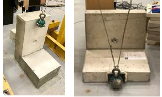
Figure 3 Small-scale pendulum impact tests for verification of new design philosophy
