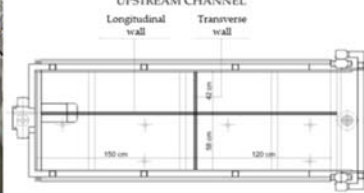
Figure 3: Detail of the upper flume, with longitudinal and cross dividing walls.
