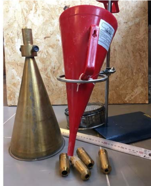
Marsh cone (funnel) viscometer 4.76, 8, 9, 10, 11, 13 mm orifice
