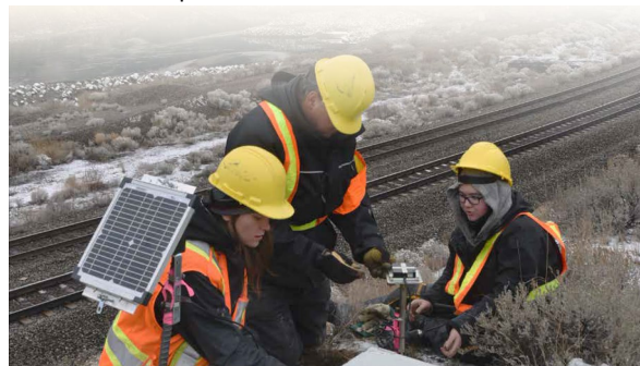
Fig.5 The GSC conducts geohazard studies to reduce risks to people and infrastructure, here installing equipment to monitor landslide activity above a critical railway corridor in central BC.
