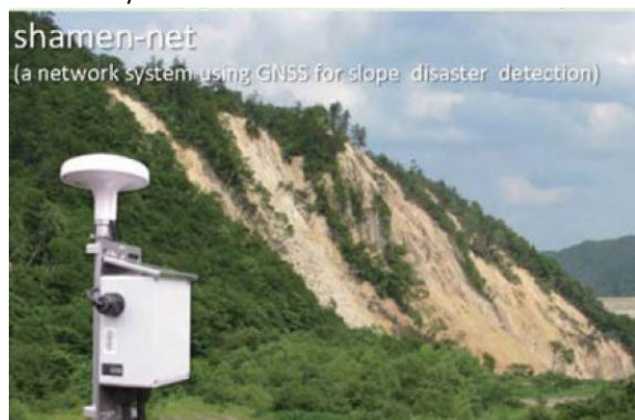
Fig 4. “Shamen-net” is a total monitoring system integrating GNSS and other monitoring device (Measurement precision: ±mm, on a real time basis)
